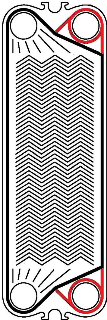
Left hand plate, periphery, material "A" Left hand plate, port, material "B"
