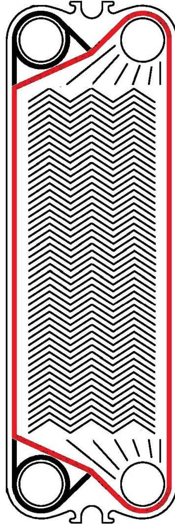
Right hand plate, periphery, material "B" Right hand plate, port, material "A"
