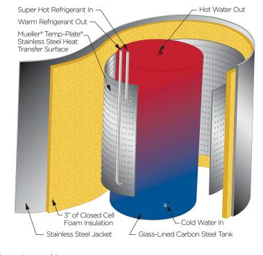
Walk-in coolers, freezers, commercial air-conditioning systems, ice machines, and other refrigeration systems all waste enough heat energy to produce hot water on a large scale. A Mueller Fre-Heater pays for itself while reducing your energy costs proportionately to your hot water usage.
